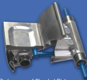
Cutaway of Pivotal Piston showing water gallery accessed via pivot shaft.
